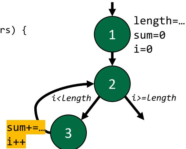
Here I've combined the increment node to keep the graph smaller
